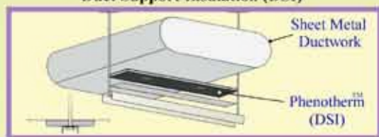
Duct Support Insulation (DSI)
