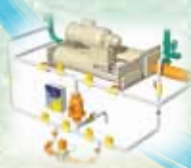
Automatic Tube Cleaning System
