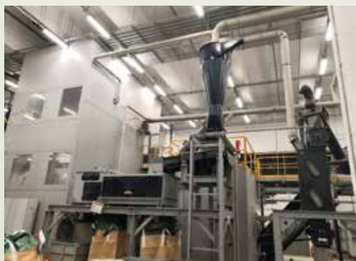
The main shredding chamber, cyclone separator and zigzag separator
